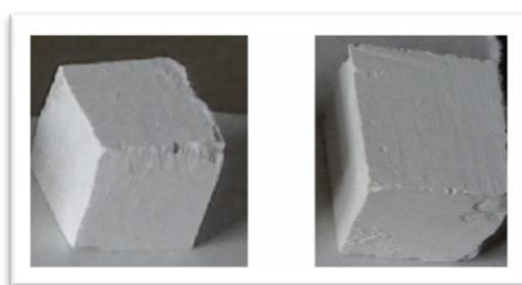
Fig. 1. Chalk stone non-treated (left) and treated with HAp (right)
